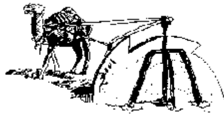
Fig.: Spiral wheel, drawing depth: 0.3-2.5 m (Egypt)
